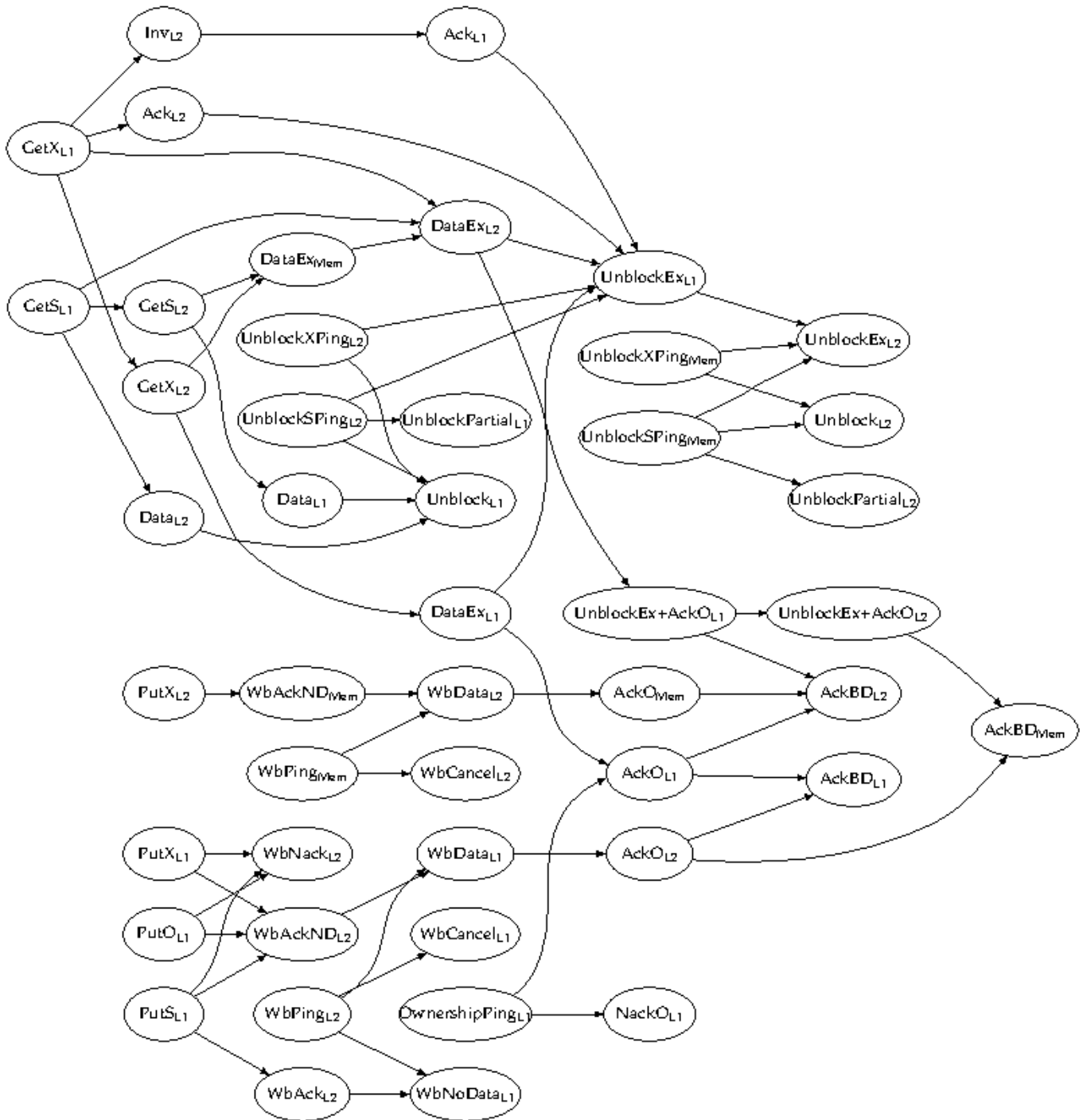
Figure C.2: Message dependency chains for the FTDIRCMP protocol
